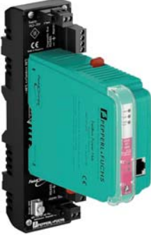
Fig. 3: the new FieldConnex Diagnostics Gateway Bus to Ethernet and detects all connected Advanced Diagnostic Modules. During setup the system configures itself.
