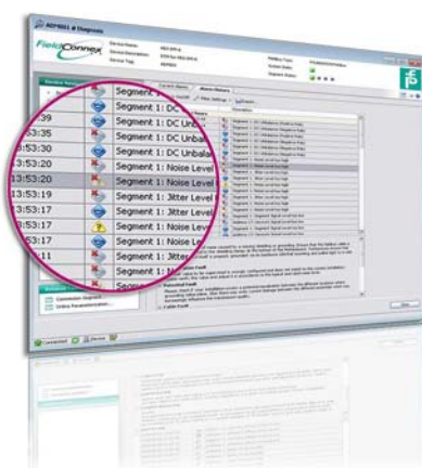
Fig. 1: Physical layer diagnostic display: Messages with time stamps and clear-text interpretation identify potential causes – powered by the built-in expert system.
