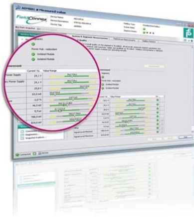
Fig. 2: Monitoring display shows all physical layer measurements in one concise display with moving sliders and memory for maximum values.
