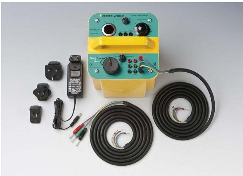
Fig. 1: Powers onsite work for a full day, recharges at night: The FieldConnex fieldbus battery including all accessories. Provides connections for fieldbus and physical layer diagnostic module. Also powers the DCS if necessary.
